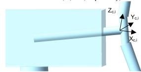
Figure 8. Coned coordinate system.
