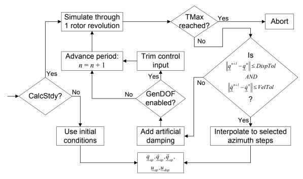
Figure 28. Periodic Steady State Computation.
