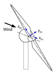
Figure 9. Blade coordinate system.
