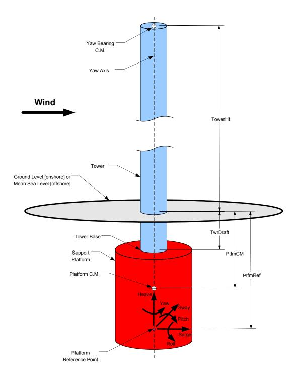
Figure 20. Support platform / foundation layout.
