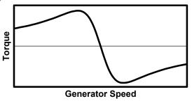
Figure 13. Thevenin-equivalent-inductiongenerator torque/speed curve.
