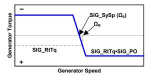
Figure 12. Simple-induction-generator torque/speed curve.
