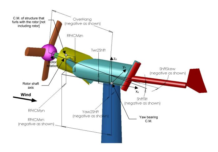
Figure 18. Layout of a three-bladed, upwind, furling turbine: rotor-furl structure
