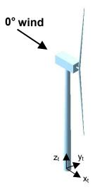
Figure 3. Tower-base coordinate system.
