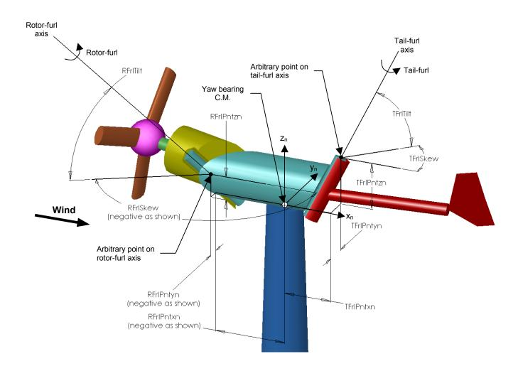
Figure 17. Layout of a three-bladed, upwind, furling turbine: furl axes.
