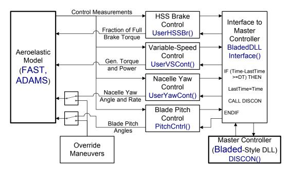
Figure 25. Interface to a Bladed-Style Master Controller DLL.
