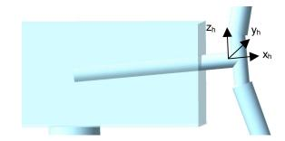
Figure 7. Hub coordinate system.
