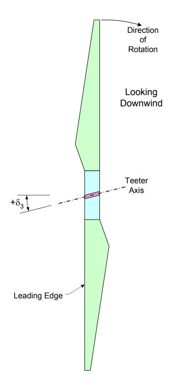
Figure 15. Layout of a two-bladed rotor illustrating  $\delta_3$ .
