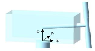
Figure 5. Nacelle/yaw coordinate system.
